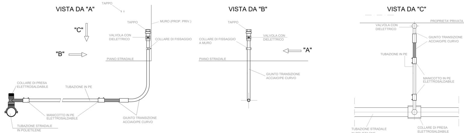
**SCHEMA TIPICO NUOVO ALLACCIAMENTO CON VALVOLA INTERRATA (PER DIAMETRI OLTRE 2")**
